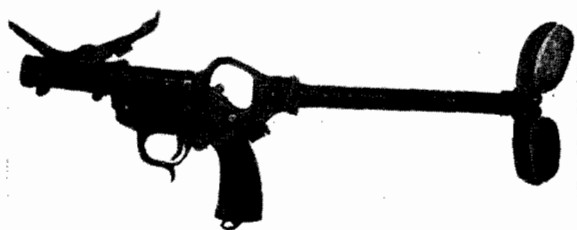
Figure 5.—Sturmpistole (modified light signal pistol).
