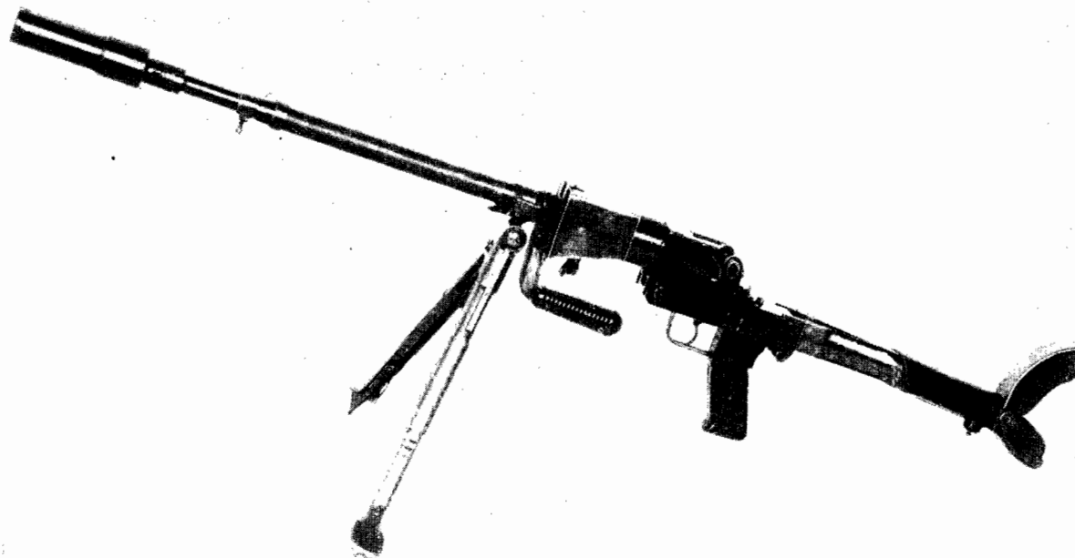
Figure 18.—Granatbüchse 39, a 7.92-mm antitank rifle modified for launching rifle grenades.
