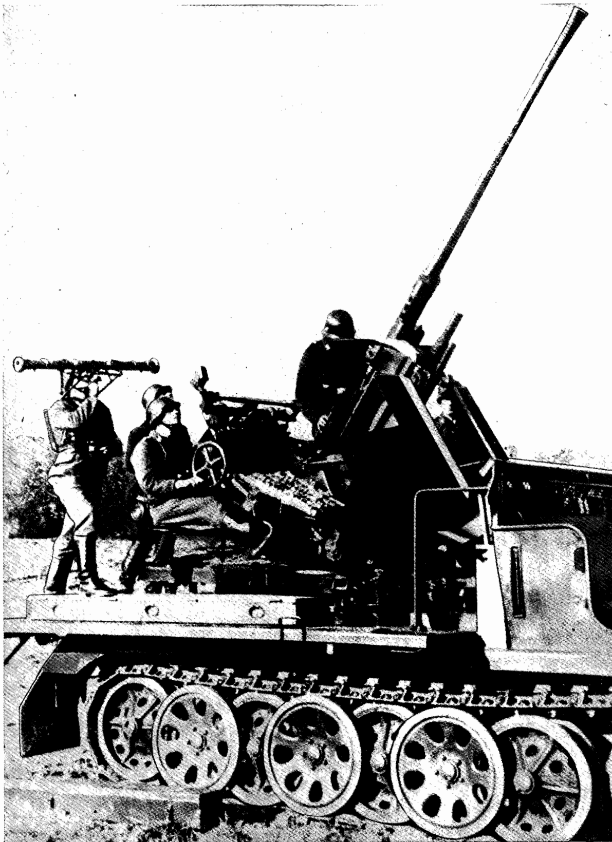
Figure 58.—3.7 cm Flak 36 (37-mm antiaircraft gun) mounted on half-track.
