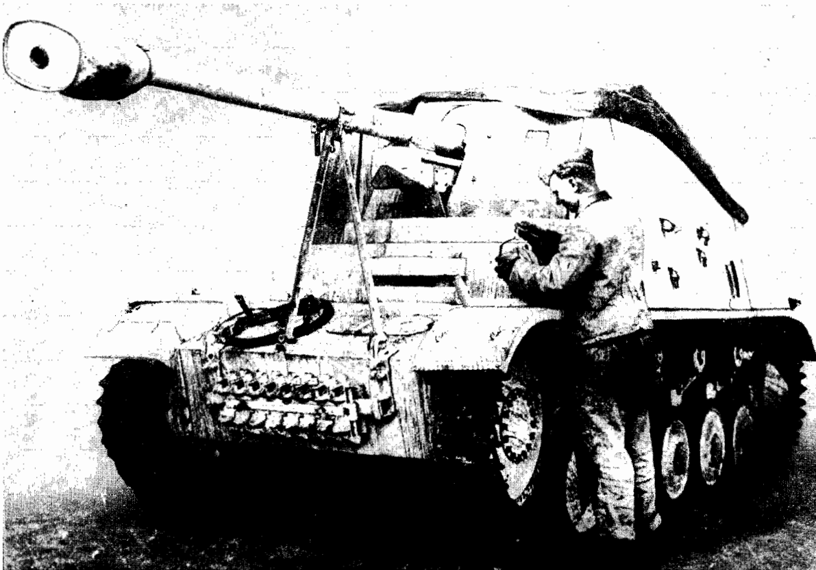
Figure 83.—7.5 cm Pak 40 on Pz. Kpfw. II Chassis.
